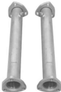
test pipes, replaces cats for track use
